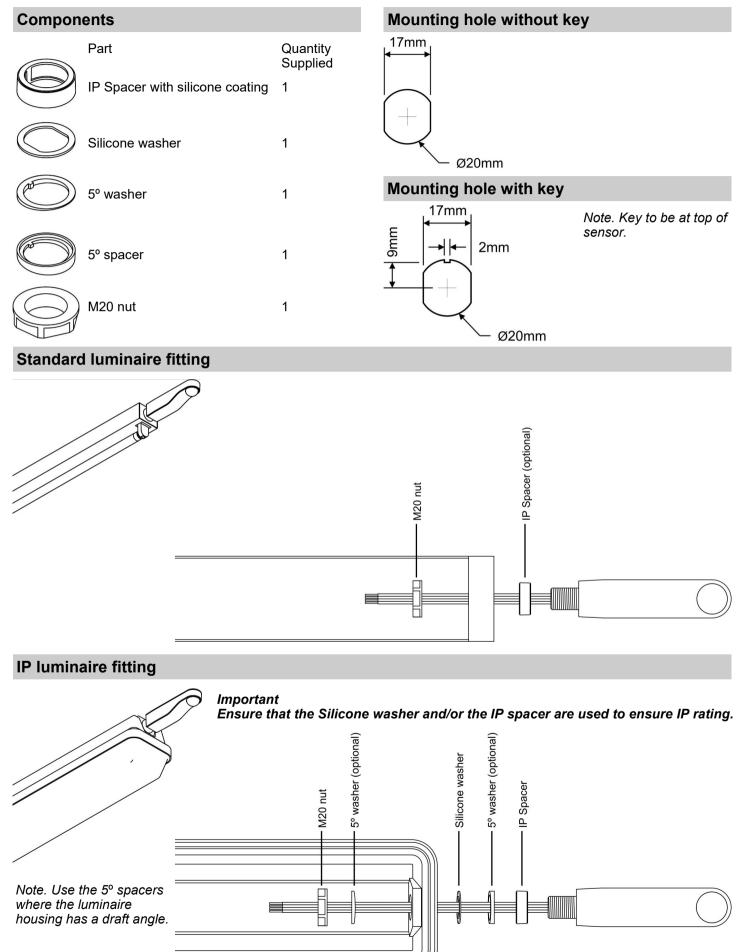
The product is designed to be mounted directly to the outside of a luminaire. The detector should be sited so that the occupants of the room fall inside the detection pattern (shown opposite), at a recommended ceiling height of 2.8m. Note that the lower the sensor is installed the smaller the detection range will be, subject to the parameters shown on the detection diagram.
